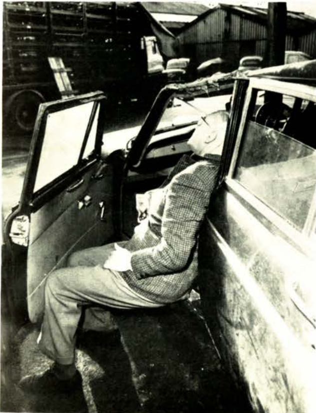
Figure 5. The single diagonal belt gives good protection, but if doors fly open its wearer can be partly ejected and catch his neck with resulting fatal or very serious neck injury.
